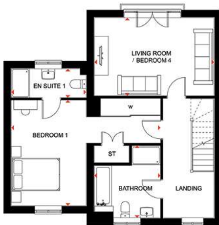
First Floor Living Room/Bedroom 4 4990 x 3244 mm 16'4" x 10'7" En Suite 1 3120 x 1200 mm 10'2" x 3'11" Bedroom 1 6225 x 4382 mm 20'5" x 14'4" Bathroom 2755 x 2996 mm 9'0" x 9'9" (Approximate dimensions)
