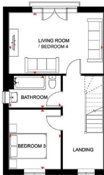
First Floor Living Room/ Bedroom 4 Bedroom 3 Bathroom 4990 x 3244 mm 2745 x 3156 mm 2745 x 1698 mm 16'4" x 10'7" 9'0" x 10'4" 9'0" x 5'6" (Approximate dimensions)
